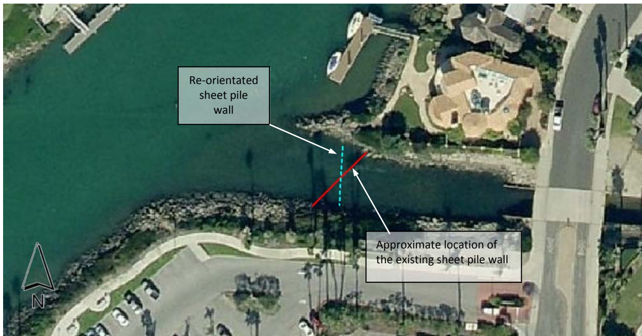
Figure 5-35. Potential re-orientation of the sheet pile at the outlet of the Arundell Barranca
