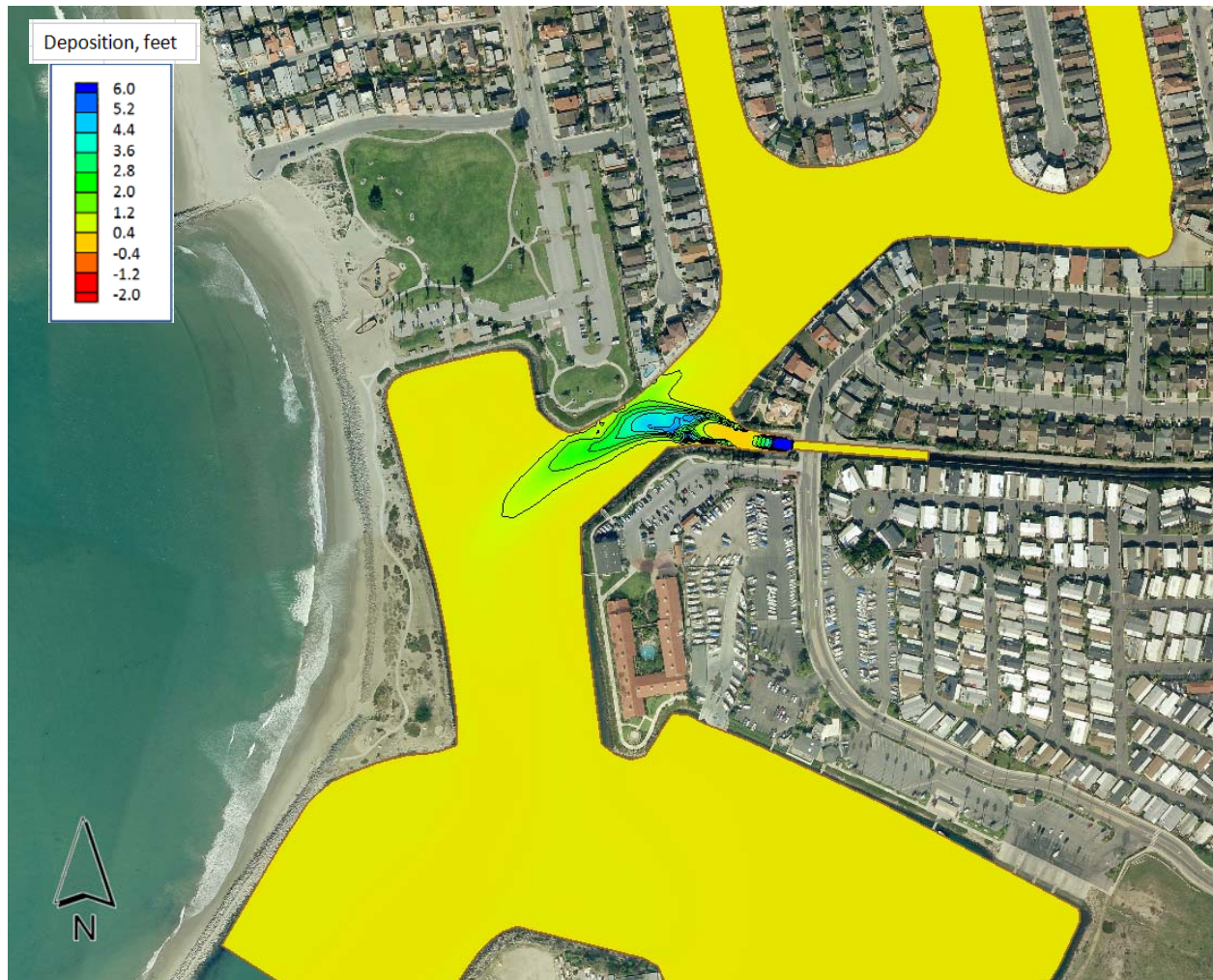
Figure 3-28. Sediment deposition resulting from 1998 high flow event for 6 February 1998 - positive values indicate increase in bed elevation due to deposition of sediment; negative values would indicate decreases in bed elevation due to erosion
