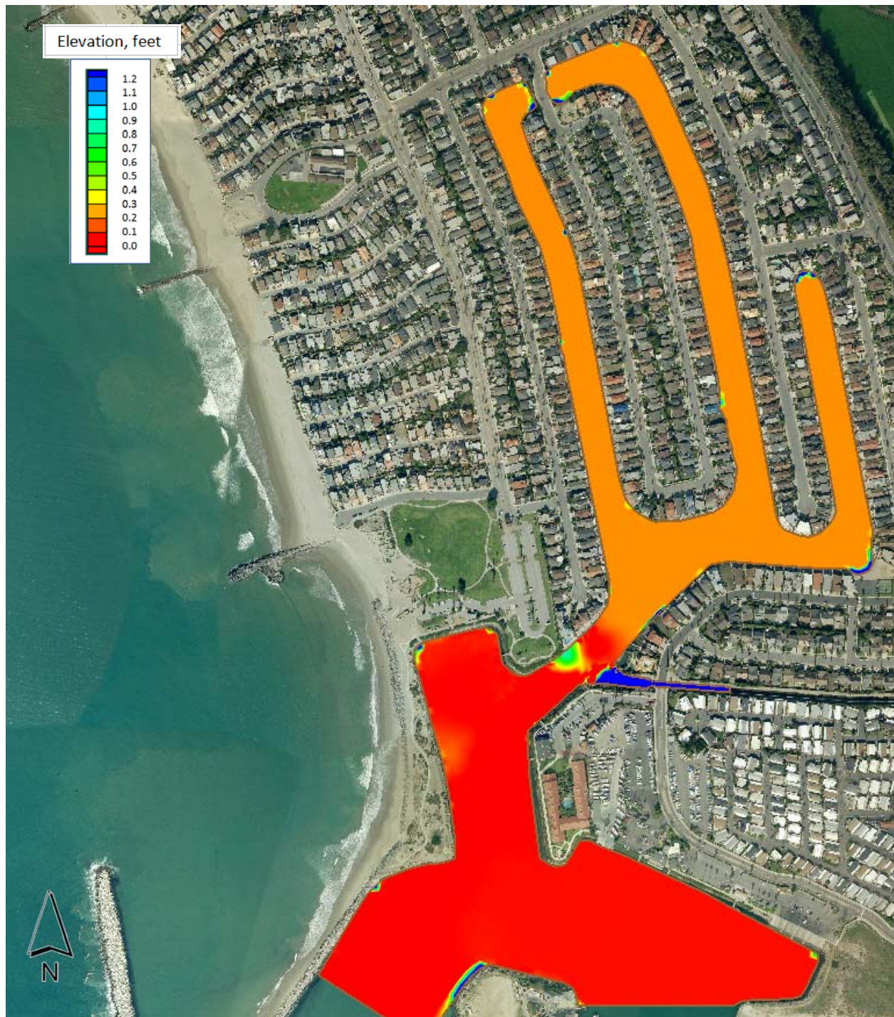
Figure 3-18. Computed water surface elevation for constant inflow of 6,000 cfs on the Arundell Barranca and tide at Elevation -0.13 ft NAVD88 (MLLW)
