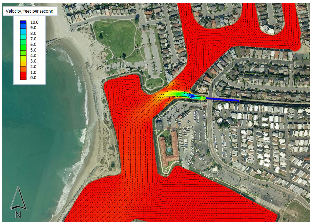
Figure 3-22. Computed velocities during 1998 storm event (Feb 6, 1998 8:50 a.m. Q=2130 cfs, Tide=3 ft NAVD88)
