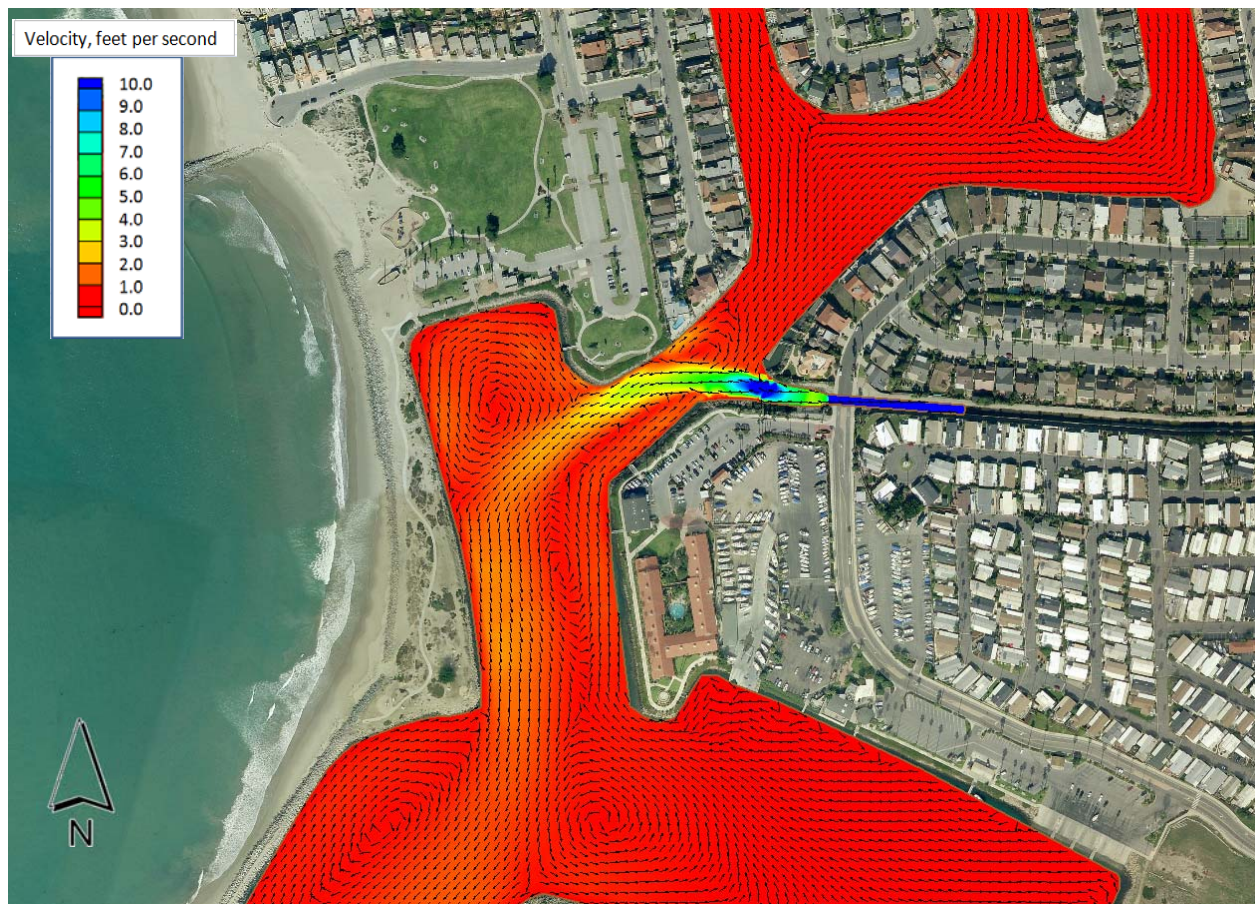
Figure 3-24. Velocities during 1998 storm event (Feb 6, 1998 9:50 a.m. Q=2020 cfs, Tide=1.75 ft NAVD88)
