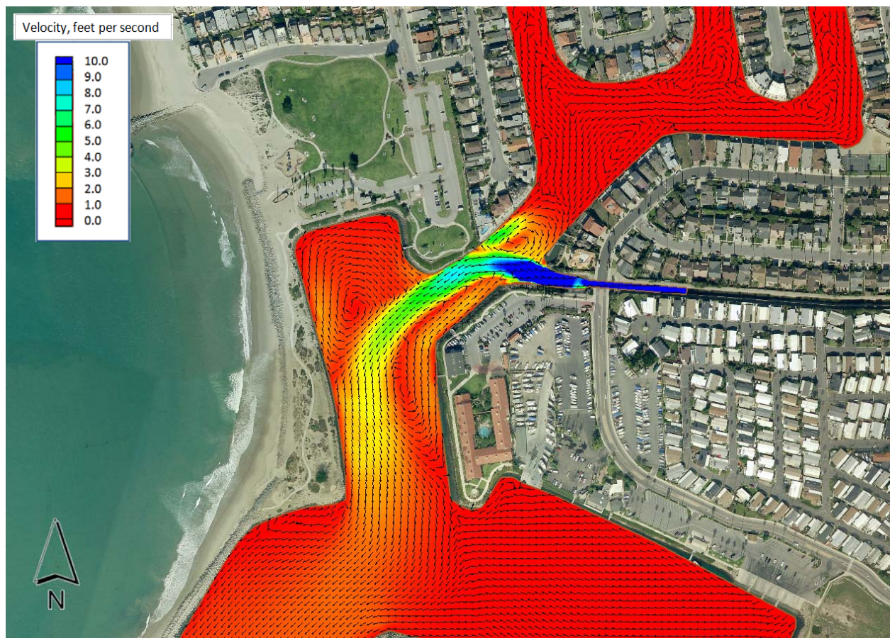
Figure 3-23. Peak velocities during 1998 storm event (Feb 6, 1998 9:10 a.m. Q=6430 cfs, Tide=2.57 ft NAVD88)
