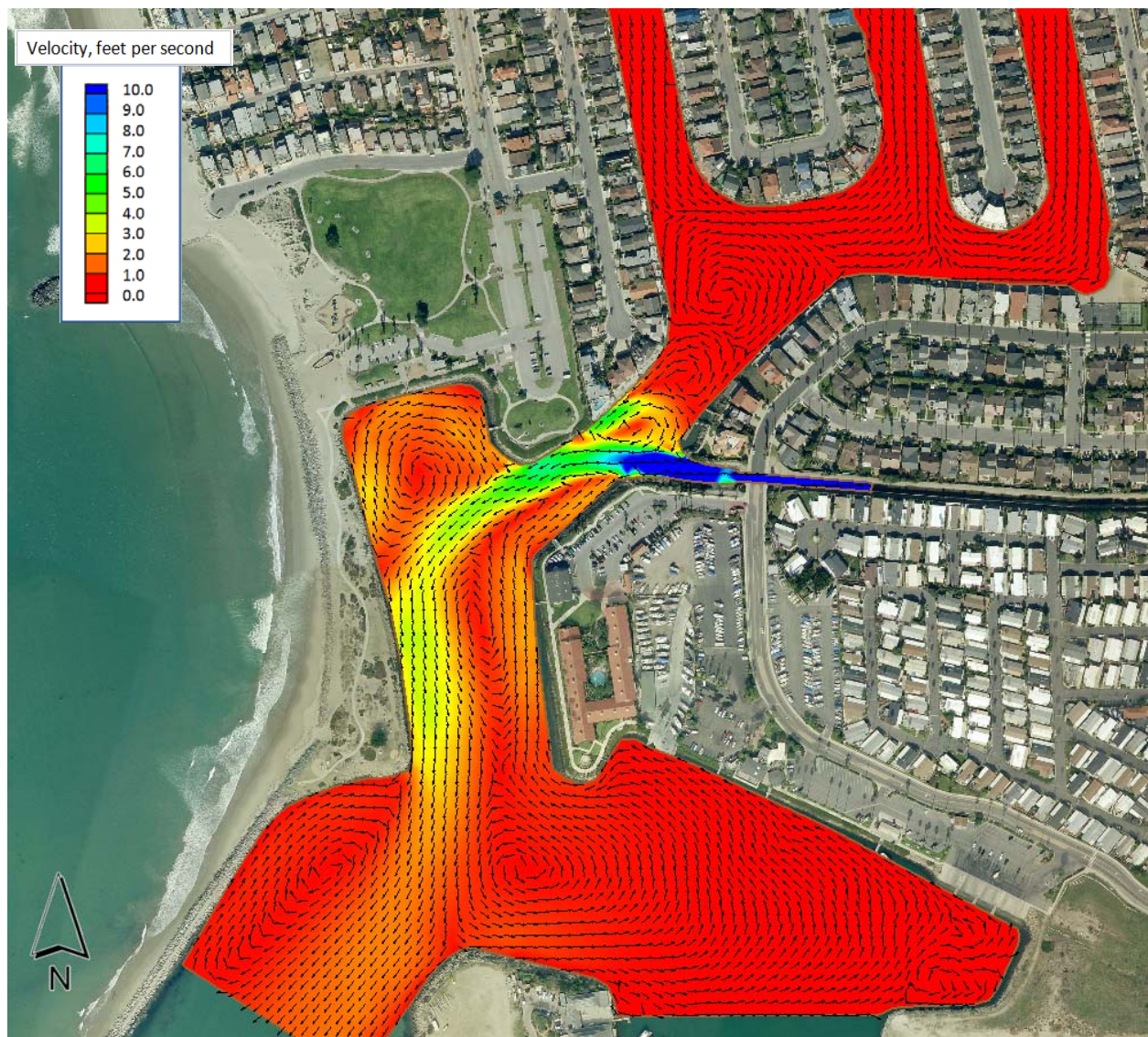
Figure 3-19A. Computed velocity at a constant inflow of 6,000 cfs on the Arundell Barranca channel and tide at Elevation 5.27 ft NAVD88 (MHHW)
