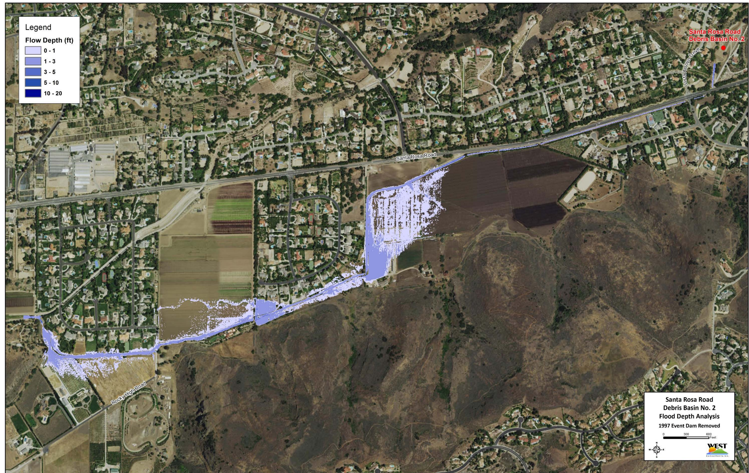
Figure D-2. 1997 Event Inundation Extent, Dam Removed.
