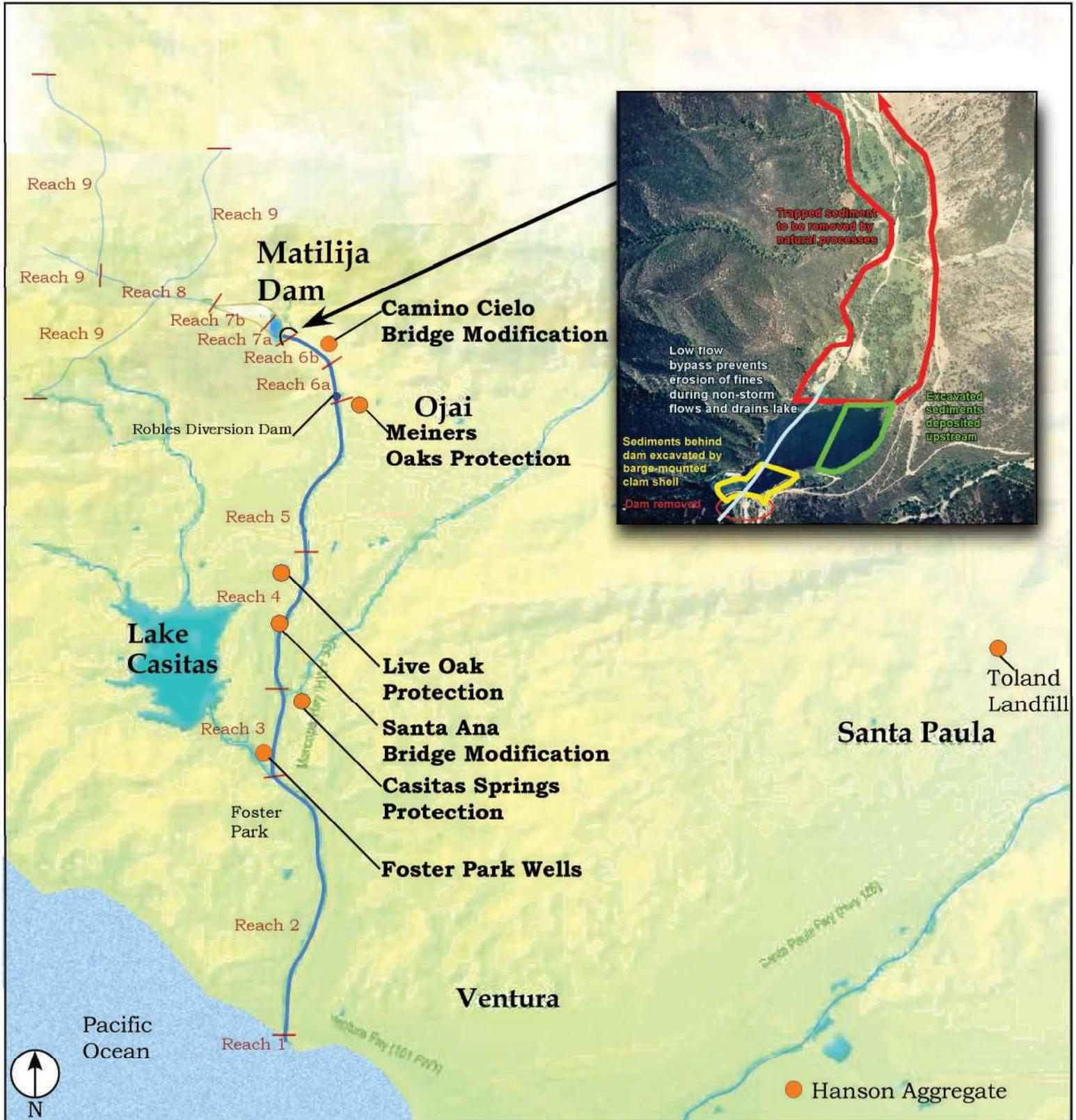
***Alternative 3a: Incremental Dam Removal/Natural Sediment Transport: Slurry 'Reservoir Area' Sediment Offsite***
