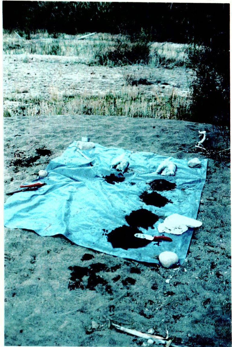
Photographs 14A & 14B. Auger site MDA-6. Photo 14A shows geologists extracting auger sample onto a blue tarp. Photo 14B shows several samples on the blue tarp. At the top of the blue tarp samples are bagged for sediment size fraction analysis and double bagged for moisture content. Photographer Joel Sturm 12/16/99.
