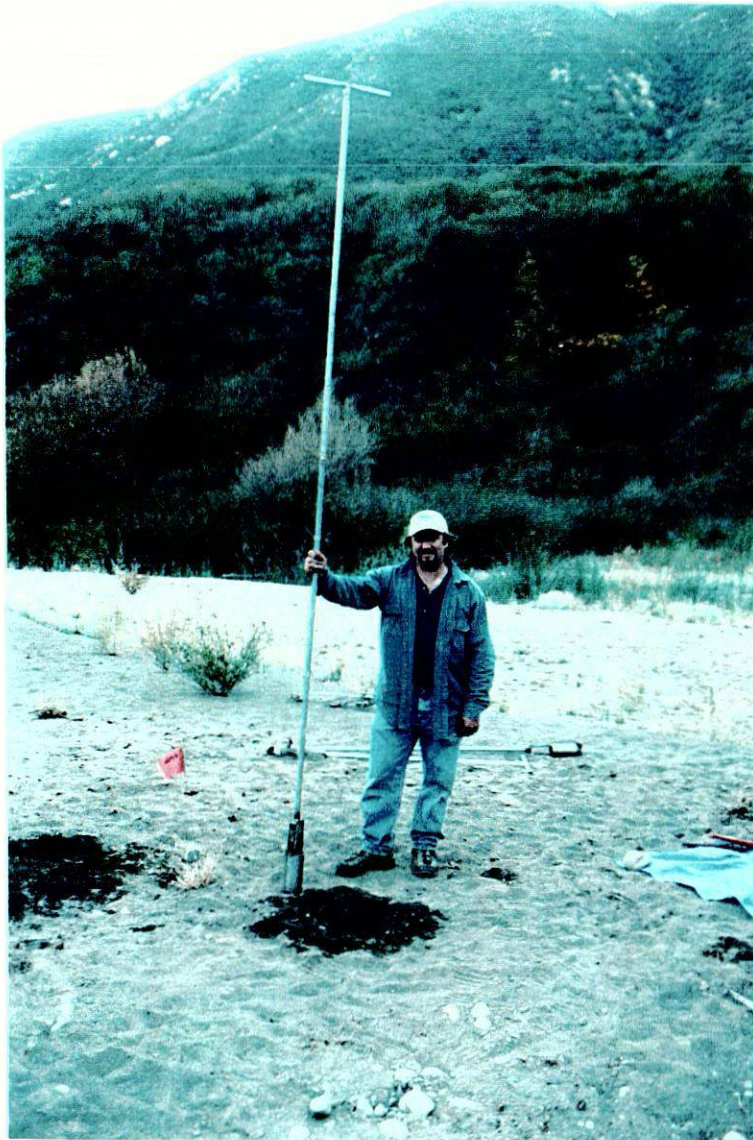
Photograph 13A & 13B. Geologists with hand auger at site MDA-6. Photo 13A shows a geologist holding the auger with 10' of rod. Photo 13B shows a geologist advancing the auger, at a depth of approximately four feet. Photographer Joel Sturm 12/16/99.
