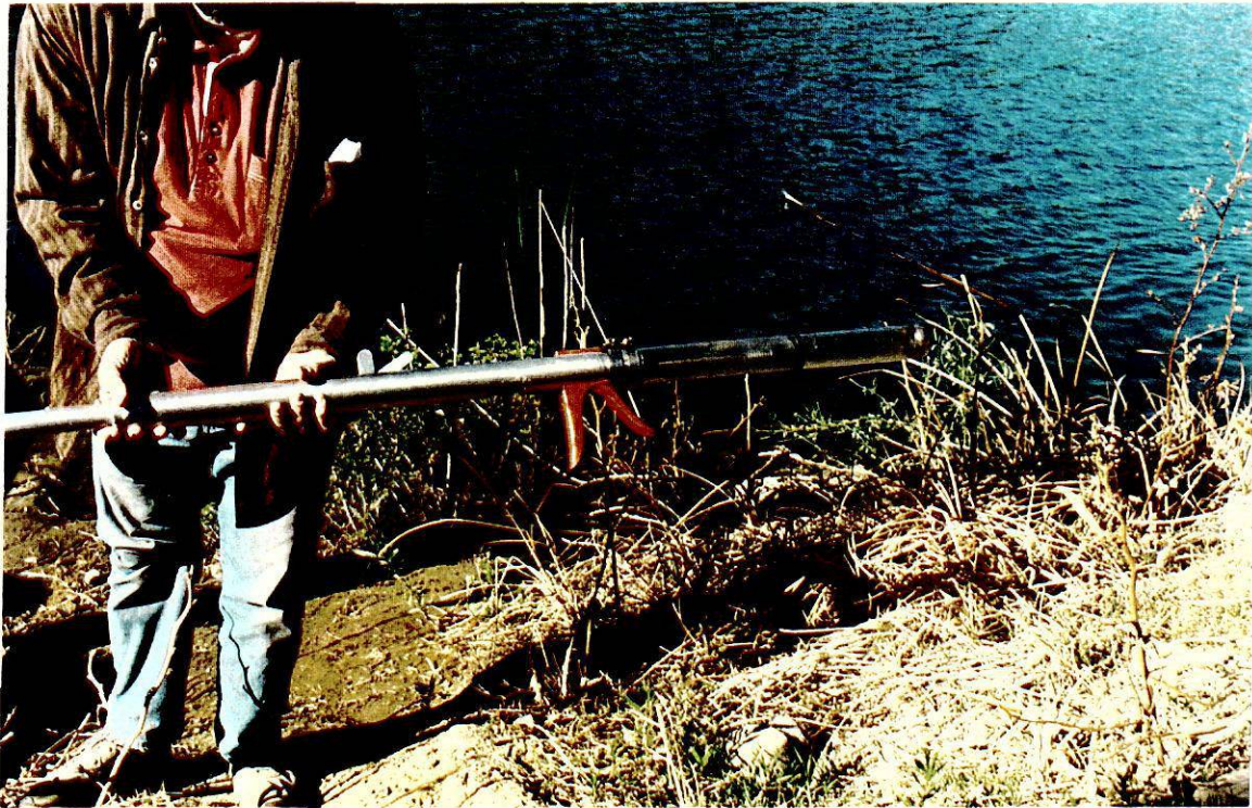
Photograph 1. View of the piston sampler used for sampling below reservoir-pond sediments at Matilija. Photographer Greg Mongano 12/14/99.
