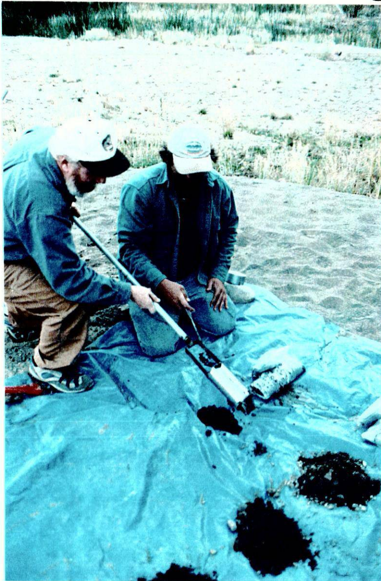
Photographs 14A & 14B. Auger site MDA-6. Photo 14A shows geologists extracting auger sample onto a blue tarp. Photo 14B shows several samples on the blue tarp. At the top of the blue tarp samples are bagged for sediment size fraction analysis and double bagged for moisture content. Photographer Joel Sturm 12/16/99.
