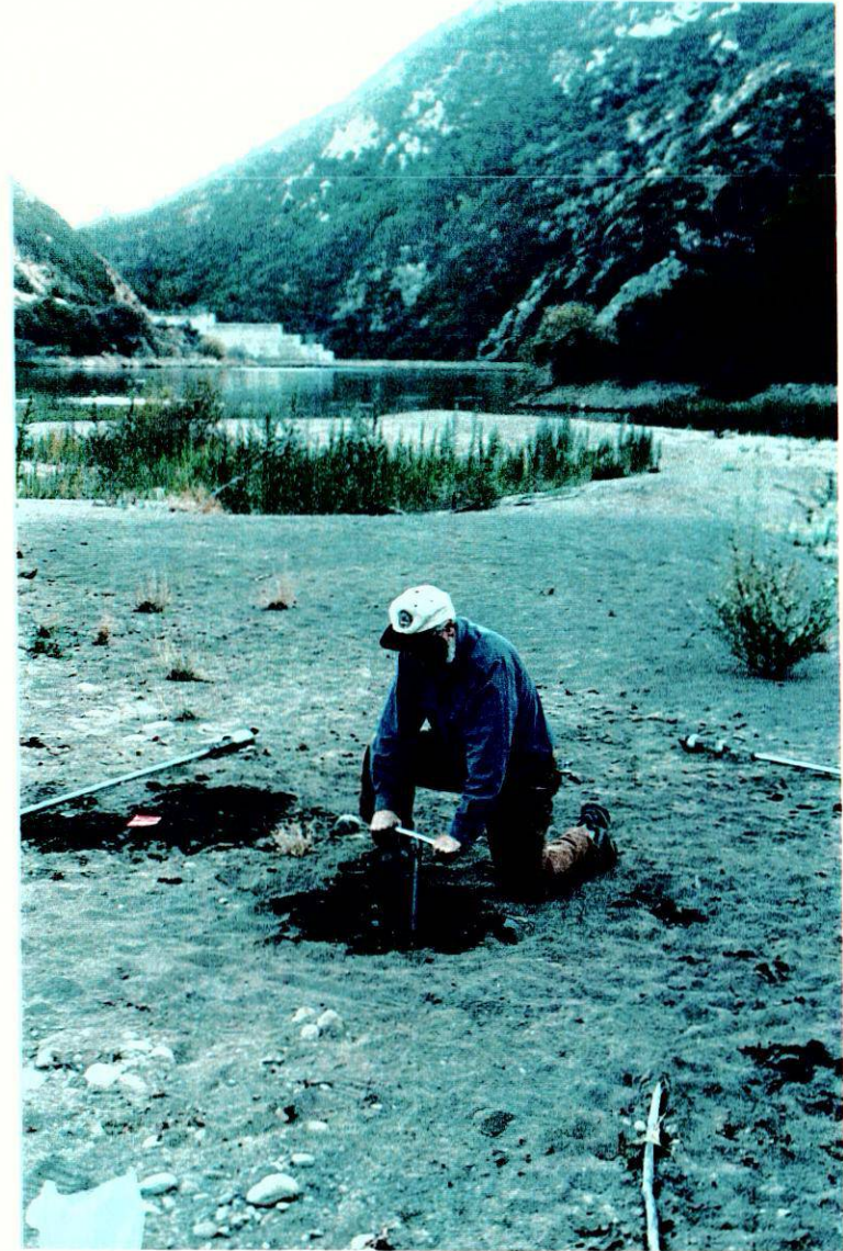
Photograph 13A & 13B. Geologists with hand auger at site MDA-6. Photo 13A shows a geologist holding the auger with 10' of rod. Photo 13B shows a geologist advancing the auger, at a depth of approximately four feet. Photographer Joel Sturm 12/16/99.
