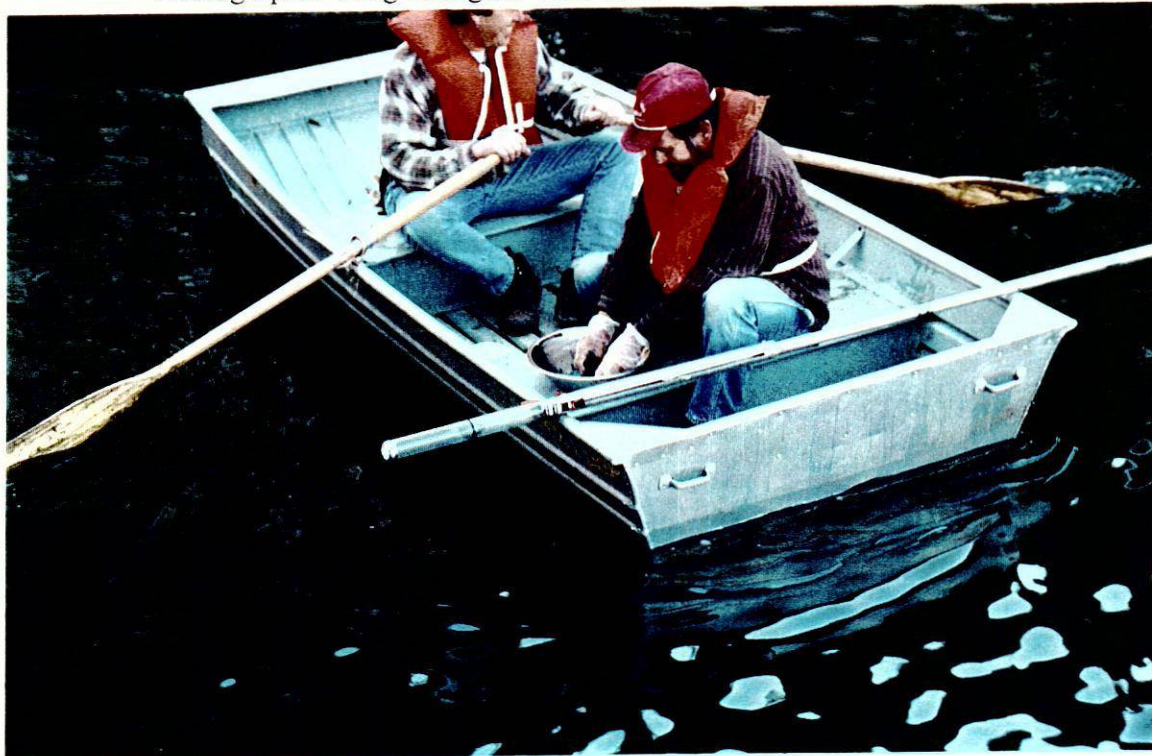
Photograph 7. Mixing of a sample collected for toxicity studies from the bottom of the Matilija reservoir pond, note the plastic gloves being used during mixing. Photographer Greg Mongano 12/14/99.
